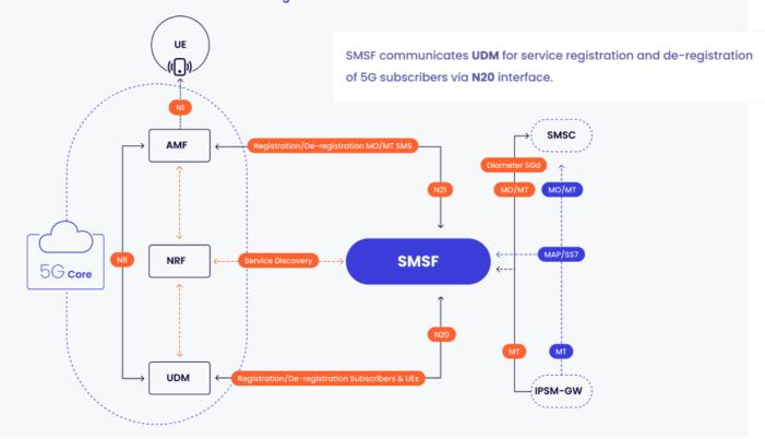
Traditional operations such as **device triggering** and **SIM OTA** will be a key feature of many IoT use cases, and operators will execute SMS delivery via SMSF. SMSF will be a key element for **Multifactor authentication** and communication with **legacy network subscribers** as well.
